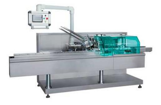
This type machine is suitable for automatic feeding and packing products into big size carton, such as food, cosmetic, tissue paper etc. This machine can automatic convey items, absorb folding carton, form and convey them, put items into carton, close and seal carton, or use glue sprayer or hot melt glue machine to seal carton according to requirement, reject unqualified product, convey finished products out.
