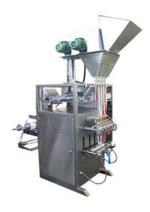
This is a fully automatic stick pack sachet packing machine for filling and sealing. It is applicable for packing powder and granular materials such as sugar, salt, milk powder, coffee powder, chocolate powder, grain powder, green tea powder, medicinal powder, nutrition powder, etc. in the industries of pharmacy, food, and agricultural chemicals.
