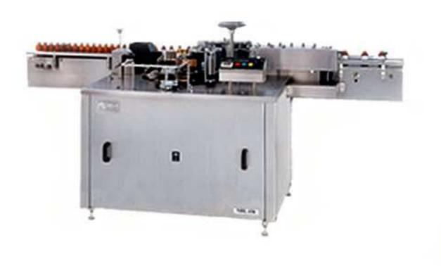
GL-80 is suitable for cylindrical container such as glass, plastic, PET bottle with paper label. The machine is economical and easy to operate. The performance is stable with a level off and good looking labeling result. The control system adopts convert motor system, the step of conveying bottle, supplying glue and sticking label automatically. This automatic labeling system is ideal for food & beverage, medical industry etc.
