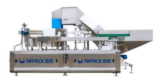
LP-200D full-automatic bottle unscrambler machine consists of elevator, bottle sorting turntable, bottle rejecting parts, bottle sorting parts, reversed bottle rejecting parts and electric box. The adjustment is simpler and the specification adjustment can be completed within 10 minutes.
