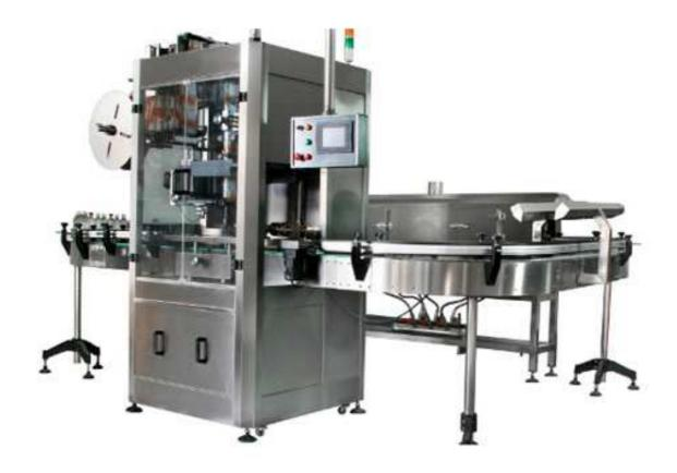
Automatic Shrink Sleeve Applicator is suitable for label sleeving in the fields of drinking, health-care products, cosmetics, washing articles for use, pharmaceuticals and petroleum and so on. Suns well Series Shrinking Label Sleeving Machines are easy to control, to change bottles and labels smoothly, and easy for cleaning and maintenance. This series machines also have a high degree of automation.
