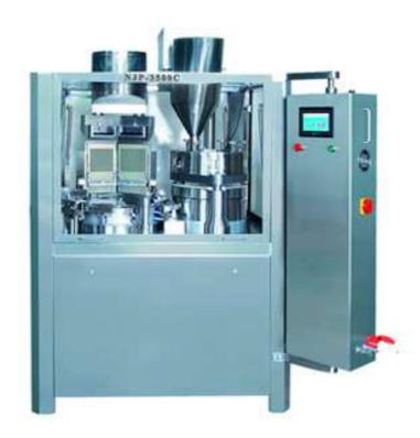
On the basis of original technology and advantages of similar products all over the world, our company developed NJP-3500 automatic capsule filling machine independently. It acquires advantages of large yield, accurate filling volume, good adaptability to medicine and empty capsules, stable operation and high automation. As a result, it can be a suitable equipment for mass production.
