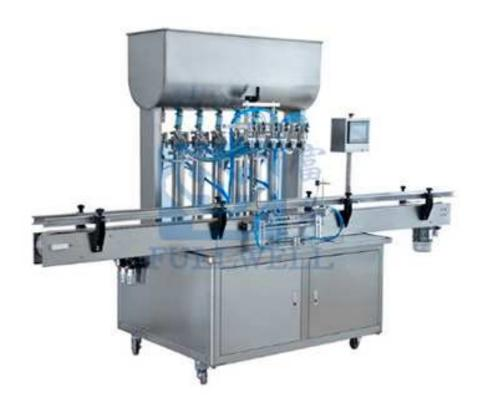
This machine is applied for viscosity and paste filling similar like juice, milk, yogurt, cream, shampoo, liquid soap, lubricant, engine oil products. It is able to integrate to capping machine and labelling machine in bottling line, fully complete and intelligence control advantage.
