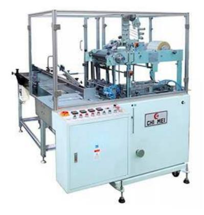
Overwrapping Machine is equipped with a "size quick adjustment system", suitable for users who often change the size of the package.
