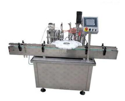
Our automatic rotary liquid filling machine adopts the brand frequency converter, with imported high-precision multi turn potentiometer and lockable dial, so that the flow regulation is stable and accurate, and the negative deviation is less than 1%, and the positive deviation is less than 1%. The stainless steel pump with magnetic gear imported from Japan has reliable quality and long service life. Stainless steel case, durable. It is easy to operate, clean and disinfect.
