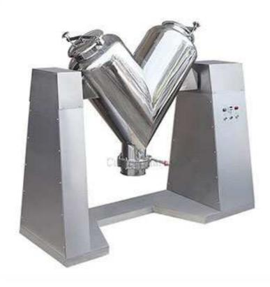
V type dry powder mixer blending machine is suitable for use in the pharmaceuticals, chemical and food industries for mixing powder or granular materials.
