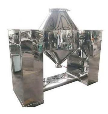
This machine adopts inside and outside rotary stirring, high uniformity. Mixing bucket can be tilted at any Angle to facilitate discharging and cleaning needs. With automatic timing device, can be set 0~60 minutes automatic stop. Using stainless steel butterfly valve discharge, no dust leakage and flying phenomenon. Using the principle of gravity diffusion mixing, the pressure feed to the material is small, will not produce shear crushing of the material.
