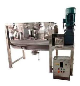
Main Application The Mixer Machine is composed of U - shaped container, spiral stirring blade and transmission parts. Spiral blade is generally made of two layers, the outer spiral material from both sides to the middle of the collection, the inner spiral material from the middle to both sides of the transmission, the formation of convective mixing. This Mixing Machine is generally used for the mixing of viscous or cohesive powder particles and the mixing of liquid and paste materials.
