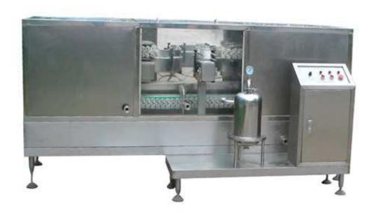
This machine is decontamination equipment of glass bottle; it is used in all kinds of cleaning of heterogeneous bottle and round bottle. Uses parallel clamps the bottle turn over transmission, and clamps the bottle caterpillar tread spacing adjustability and the reliability; Each bottle can pass trough multi-channel returns the water used, the pure water and purification compressed air clean processing, achieves the ideal clean effect.
