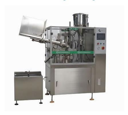
ZHY-60YP plastic tube filling machine is broadly used in cosmetics, light chemical, pharmaceutical, foodstuff and other industries. Such plastic tube sealer is suitable for packing ointment, cream, gel and sticky fluids. Plastic, plastic composite and aluminum plastic composite tubes are available.
