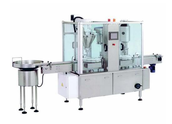
The Automatic Cap Sealing Machine is designed for automatic filling medicine into bottle (small volume) and cap sealing, such as Chinese herbs powder, dry syrup powder and aerosol powder etc.
