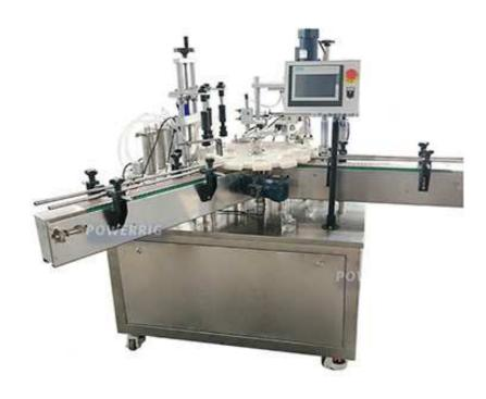
A semi-auto soft glue filling and capping machine is mainly used for glass bottle perfume filling and capping.
