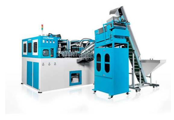
A handle bottle makes it easier to carry and pour from a container to container. CMS series stretch blow molding machine equipped with a robot device is the choice of making bottle with handle. The container with a firmly fixed rigid polypropylene handle ensures the shape that does not been distorted, and it is currently used for new products, especially for family size packs.
