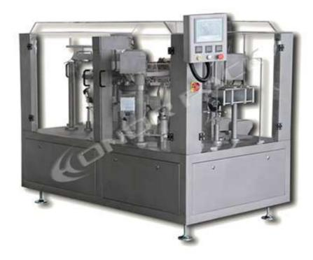
It is the bag clamping that is specially used for spout bags. It is equipped with horizontal bag sending device and high speed free flowing/ viscous liquid, which are specially used by spout bags. This makes packing speed of spout bag up to 35 bags/min.
