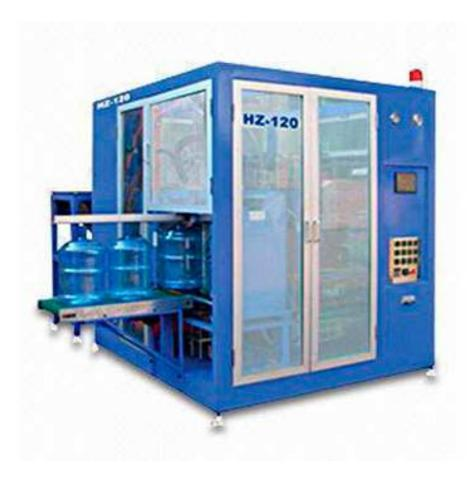
HZ-120 automatic PET stretch blow molding machine, PET bottle blower is used to produce five gallon (20L) PET bottle, nowadays 20L sized bottles are demanded extremely in the market. Facing great demand for 5 gallon PET bottle at market, the whole bottle making production from perform conveying to bottle discharge is completed automatically. It is made up with three main parts: perform loading system, Heating oven & blow station.
