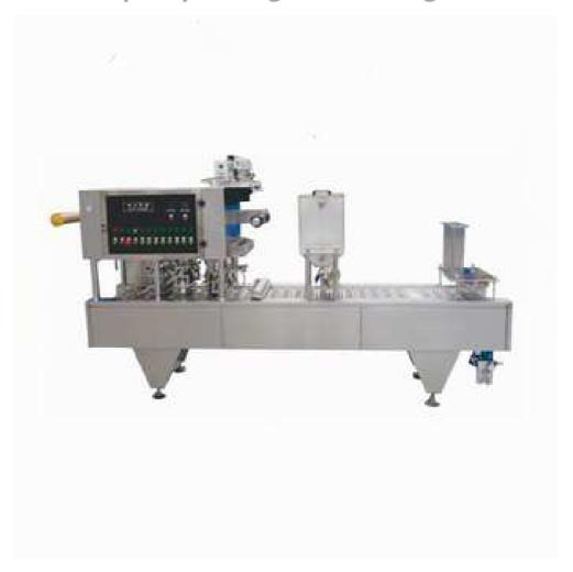
This series is widely used in various kinds of plastic cup for liquid filling and sealing. It can automatically finish the process of filling, sealing, cutting, printing the code, sterilizing in ultraviolet radiation and falling cup etc.
