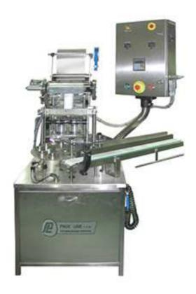
This semi automatic sealing machine features a rotary system and may include outlet and inlet containers that make it easy to transform to automatic mode.
