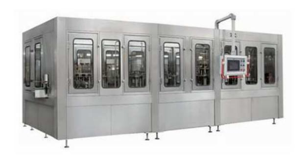
Automatic Juice Filling Machine for pet bottle and glass bottle is widely used in production of drinks, including fruit juice filling, soda drinks, beverage filling, and carbonated water filling and so on.
