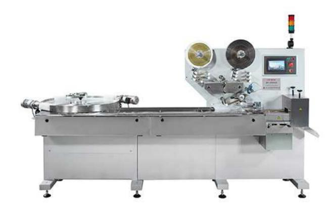
The JH-Z1205 is a horizontal high-speed wrapping machine for hard candy in fin seal (pillow pack). The products are transferred by the removal wheel and delivered to the segments of the cam chain. Two pairs of sealing rollers for the longitudinal seam and a cross sealing unit guarantee a tight pack. The standard version is equipped with automatic splicer to change wrapping material reels without stopping the machine.
