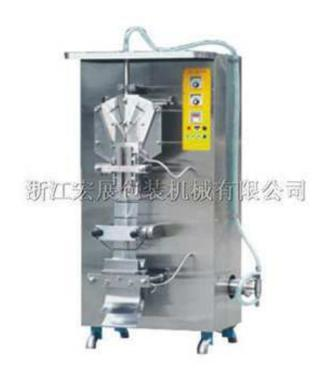
This machine is widely used to pack liquid of low and high viscosity such as pure water, milk Juice, beverages, soy sauce, vinegar and wine. It can automatically sterilize the film with violer ray, form the bag, print the code precisely, fill the product and seal cut at one time. Model HP1000L-I and HP1000-II used single lay PE film and co extrusion film and the HP1000L-111, HP1000L-B used printed laminated film such as PET/PE, OPP/PE, to present more attractive packing.
