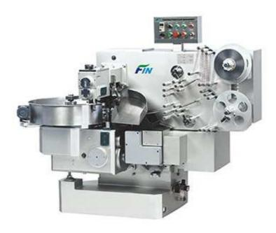
Double twist packing mainly applied for milk candy, peanut candy, chocolate, etc. The feeding plate has the connector to install auto hopper device.
