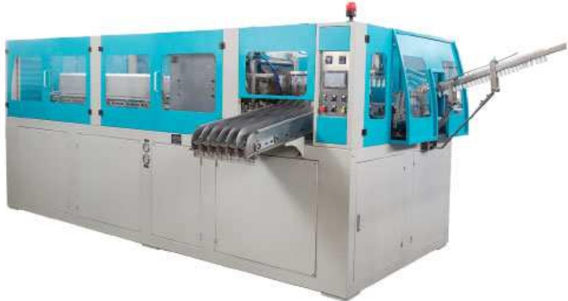
The conveyor put the preform from the barrel to the entire machine, then the preform is automatic arranged in order to feeding in a single way Adopt FESTO rodless cylinder to divide into blank movement and positioning. The clipper picks preforms is place them on the transfer system. The way will avoid preforms jamming or wasting preforms.
