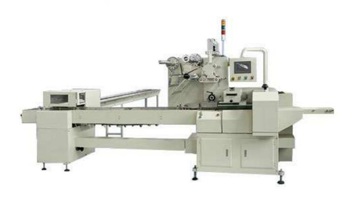
FWL280B On-Edge Biscuit Packaging Machine is specifically applicable to wrapping group biscuits standing vertically on edge.
