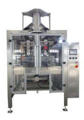
Automatic bag form-fill-seal packing machine explores the roll of film to make bags of pillow bags, gusseted bags. The maximum film width is 1100mm. Large loading weighed can be added which is up to 20kg. It can automatically realize bag making, filling, printing, sealing, gusset making, hand hole making, etc.
