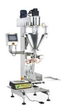
This machine is a semi-automatic series filling and packing machine Horizontal bin opening Machine interface, PLC weighing module control Servo motor drive screw, 304 stainless steel, suitable for Artificial bagging.
