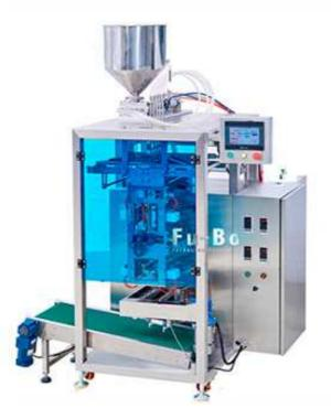
PLC Controlled, equipped with piston pump filling system. Applicable for the liquid/sauce package.
