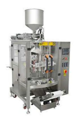
Packing Machine PL-420YB is suitable for packing liquid products such as water, oil, sauce, etc.
