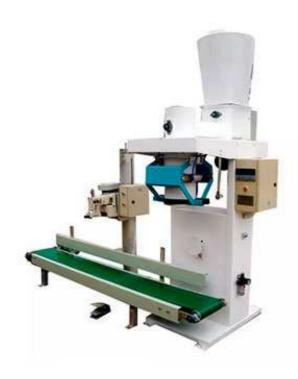
Mainly applicable to powder material (flour, bran, starch, feed, chemical powder etc.) similar materials.
