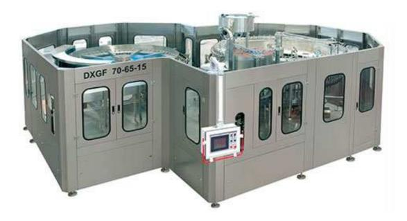
Carbonated beverage filling machine is mainly used in carbonated beverage production line. It adopts PLC to control the whole machine operation. This machine is suitable for bottled soda water, carbonated beverage product, etc with production capacity ranges from 4000BPH to 36000BPH based on 500ml volume.
