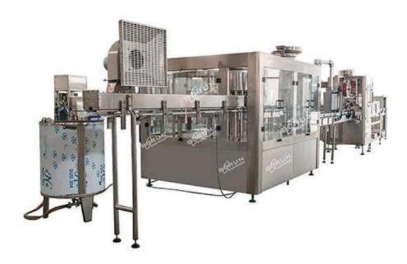
Automatic drinking water bottling machine combined water bottle washing, filling and capping into 3 in 1 monoblock. It is suitable for both plastic polyester bottle (PET bottle) and glass bottle with screw caps for non-aerated carbon dioxide drinks such as mineral water, pure water, non-gas water, spring water and so on. The water filling machine design could shorten the time for the drink material contact with outside, increase the sanitation condition through economy benefit.
