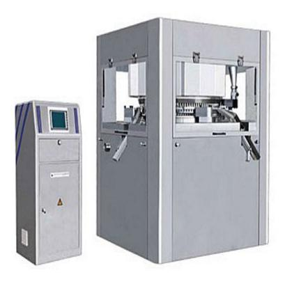
The first triple sided tablets press in China, 3 separate filling stations, servo control filling, and feeding powder in 3 hoppers - cancel hydraulic system. Use mechanical support for compression roller is controlled by motor with a encoder.
