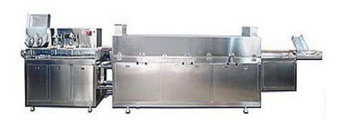
This machine applies the high-precision orientation screen board print. Control system applies the programmed controller. Agglomeration subsection control temperature.
