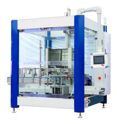
It is used for the carton packing and work with the logistic code system. This carton packing machine is widely used in the food, daily products, agrochemical and other industries.
