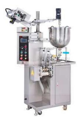
Liquid Packing Machine is automatically filling and sealing for packages of liquid products such as sauce, milk, oil, honey, ketchup, jelly, peanut butter, also the cosmetic products like shampoo, conditioner, lotion and hand cream etc. Operating with the rotary pump with servo motor dosing in high accuracy and high stability.
