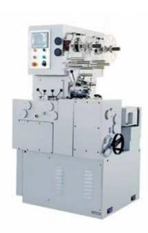
Twist Candy Wrapping Machine is suitable for double twist packaging of candies (with different kinds of shapes like rectangular, oval, circular, cylindrical, square), chocolate, beef granule and so on, with single layer or double layers wrapping materials.
