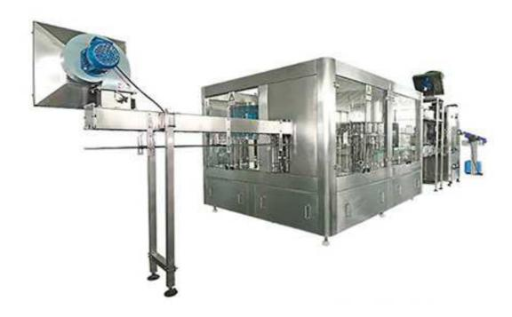
Automatic machine for bottle washing filling and capping, with 18 washing chucks, 18 filling valve and 6 capping heads, production capacity for 500ml mineral water is 4000 bottles per hour. The available bottle sizes for this machine are 300ml – 2000ml.
