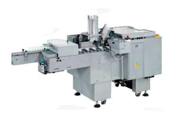
This machine completes product insertion, leaflet insertion and production batch & expiry date coding in one run. Also equipped are malfunction warnings for fail safe packaging processes. It is labor saving, suitable for pharmaceutical, ointment or cream tubes, cosmetics, hardwires, stationary, etc.
