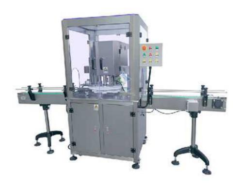
Automatic ring-pull cans sealing machine is suitable for the sealing of various tin cans, tin cans, aluminum cans, paper cans and other round specifications. It is easy to operate and is an ideal sealing machine for food, beverage, pharmaceutical, chemical and other industries.
