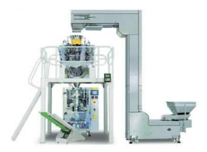
Z520 combined weighing type full automatic particle packing machine has two kinds: carbon steel type and stainless steel type to meet customer's various needs. Z520 full automatic particle packing machine can automatically complete material upper feeding, weighing, packing and conveying. This combined weighing packing machine includes:
