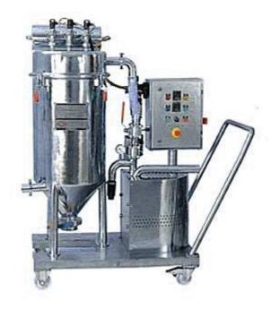
PMS Vacuum Feeder® provides the unique pneumatic-transferring system of the dry solid particles in the close system. It significantly reduces the conventional material handling, as well as, completely eliminates the risk of contamination. The usual bulk density for the material to be transferred should be less than 0.5 kilogram per liter and the distance of vacuum system should be less than 50 meters.
