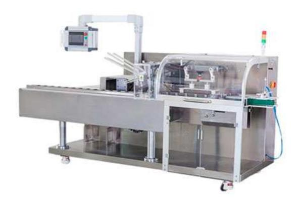
The product is unloaded according to the specified arrangement, and it automatically enters the sorting point mechanism. After the point is completed, the product enters the synchronous belt of the cartoning machine. With all the functions of pushing, inserting and sealing, the machine is estimated to save six people and increase production efficiency by about 1.5 times.
