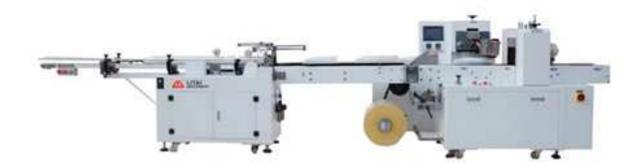
This cup packaging machine adopts touch screen, PLC, servo motor drives two-way to count cups. All imported components and parts choose international famous brand; The body is of compact construction. It can reach the advantages of stable performance, high precision, fast speed and simple operation.
