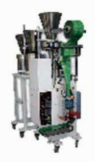
The machine is composed of volumetric conveying cups, vibration device and convey. The volumetric conveying cups are used to convey and measure free flowing products like beans, powdered soup, salt etc. The bowl vibrating feeders are used to convey irregular products like lump meats, dried shrimps and so on. The bucket conveyers are used to fill multi-products into one bag
