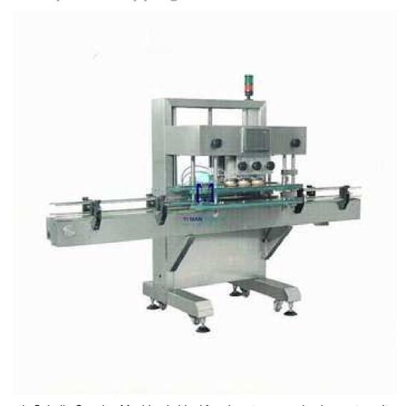
The Automatic Spindle Capping Machine is ideal for almost ever packaging system. It provides continuous capping for a wide variety of cap sizes, cap types, container sizes and types. It is flexible and durable, ideal for both in-case capping, and on-line capping.
