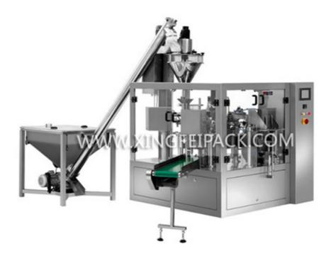
Automatic Premade Pouch Filling and Sealing Machine is used for the flat bag, standup bag, bag with zipper.
