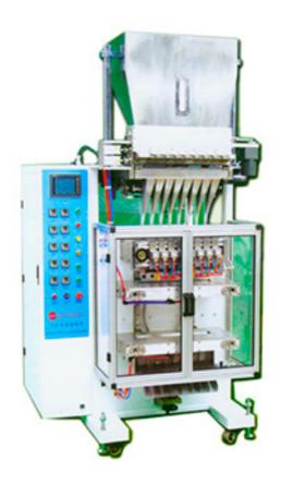
KDL multi-lane automatic packaging machine adopts bar pillow sealing type. Bag looks nice. Apply for the granular packing in the industry of foodstuff, medicine, chemical and so on. Use this model can save manpower, improve efficiency of production and suitable the standard of sanitation.
